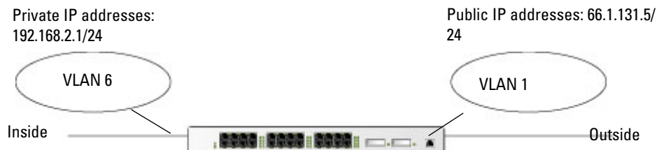
Figure 4 Example: Source NAT using Controller IP Address
